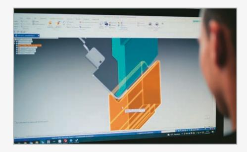
Our bending simulations give you a realistic overview of our 3D bending process, showing any collisions that may occur during the process.
